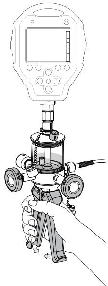
Repeat step 6 while connected to the Device Under Test until no bubbles escape the Fluid Return Hole.
