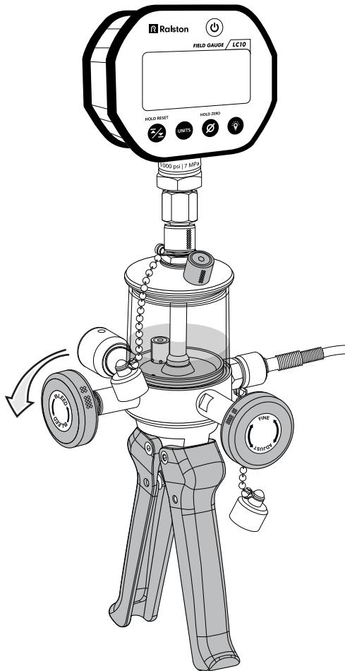
When finished testing, open the bleed valve and vent the remaining pressure from the system.
