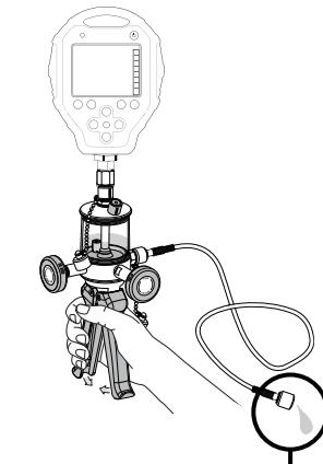
Pump hand pump until fluid comes out of the end of the pressure hose.
