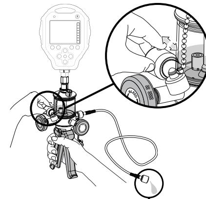
Pump priming piston until fluid comes out of the end of the pressure hose.
